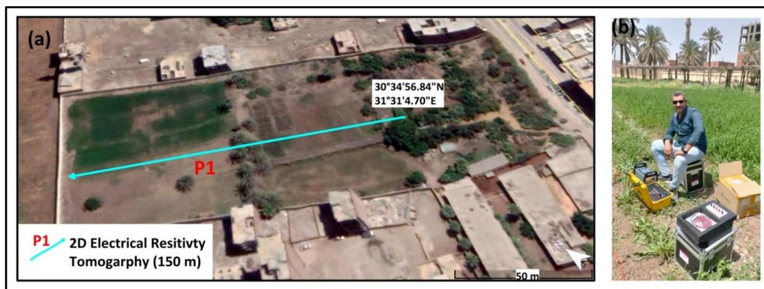
Fig. 1: (a) Location map of the study site showing the 2D-ERT profile (P1) and (b) Field photos showing the field data acquisition using Geomative GD-20 resistivity meter at the study site.
