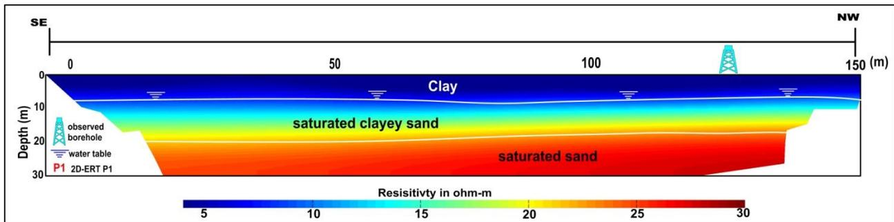
Fig. 2: 2D interpretation of the 2D-ERT P1 (for location, c.f. Fig. 1a), obtained from inversion of Wenner data set.
