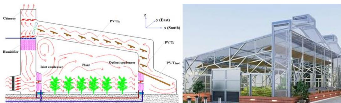
Figure 1. Conceptual configuration of the solar driven greenhouse, 2-D (left [1]) and 3-D (right)
