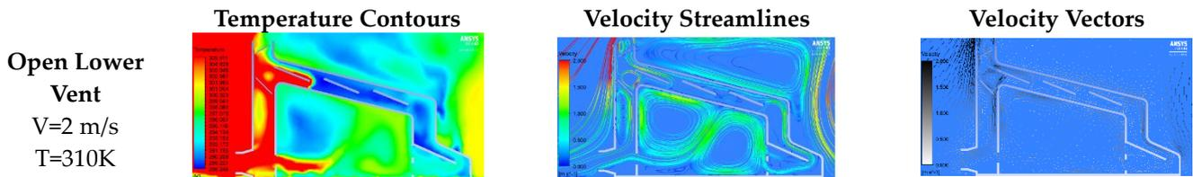
Figure 3: Temperature contours, velocity streamlines, velocity vectors for open lower vent scenarios with the initial conditions of velocity 2 m/s and temperature 310 K [2]
