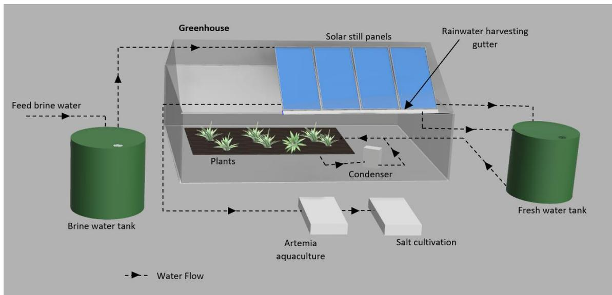
Figure 1. Conceptual model of the zero liquid discharge and desalination system
