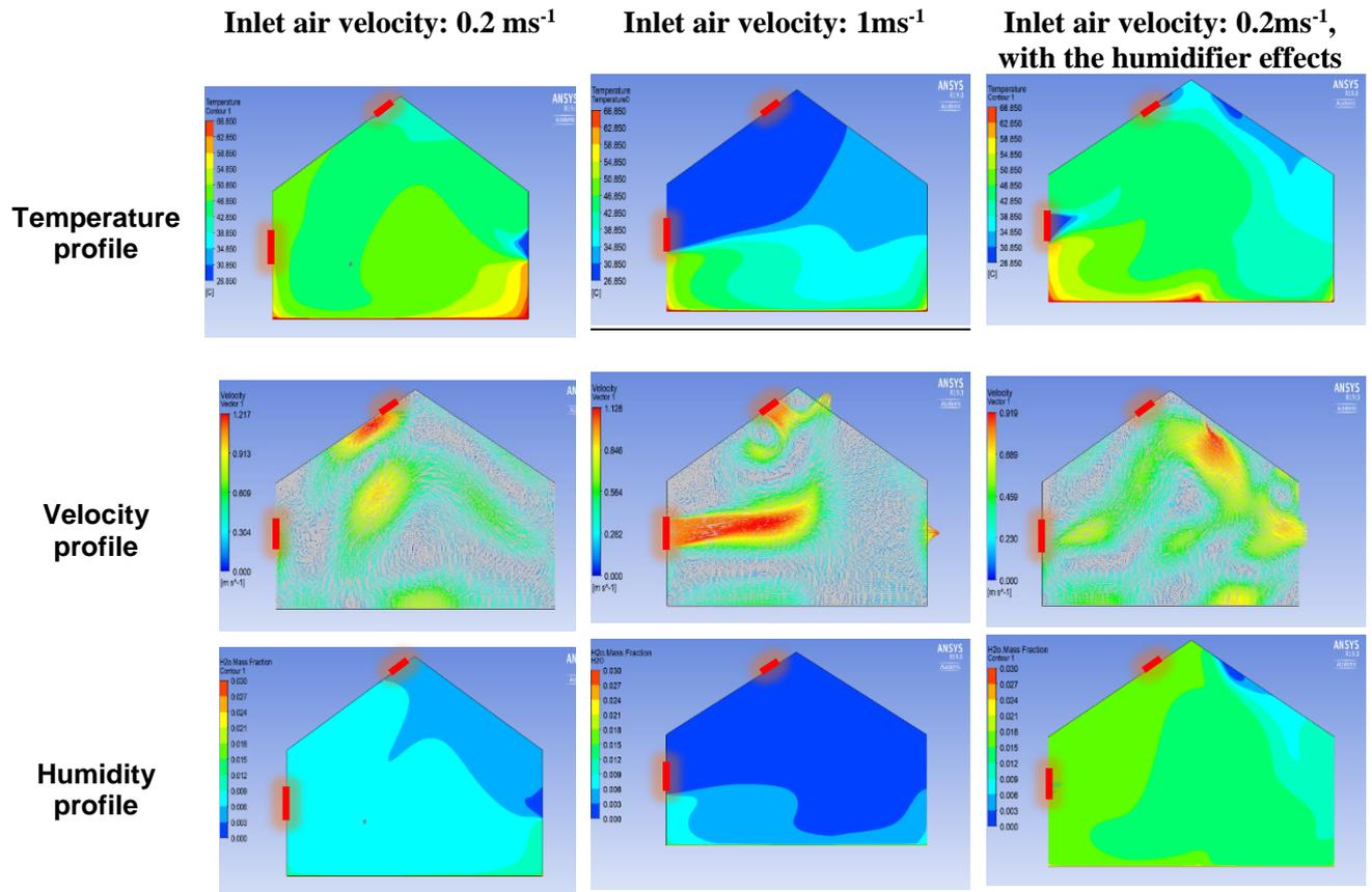
**Figure 1:** Inlet wind velocity effects on the temperature, velocity and humidity profiles
